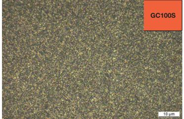
GC100SN Classification K20/K40, Buick C1, (C10 + C5 Coated) Ultra fine grade with maximum toughness for rotating tools, especially for roughing applications.
